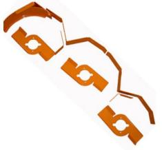
The "Eye of the Hurricane" mulch plates efficiently force the cut grass into the path of the Eliminator blades, where it is shredded and quickly driven into the ground. This prevents loading up of grass clippings on the underside of the deck and requires less horsepower to mulch, even in moist conditions.
